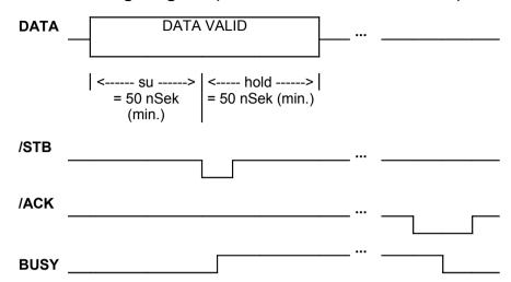
su = Set-Up-Time Data valid until /STB LOW = 50 nanoseconds (min.). hold = Hold-Time /STB LOW until DATA changes = 50 nanosesconds (min.). /STB-width = 20 nanoseconds (min.). /ACK-width = 0.5 microseconds (nominal). /STB LOW until BUSY HIGH = 40 nanoseconds (nominal).
